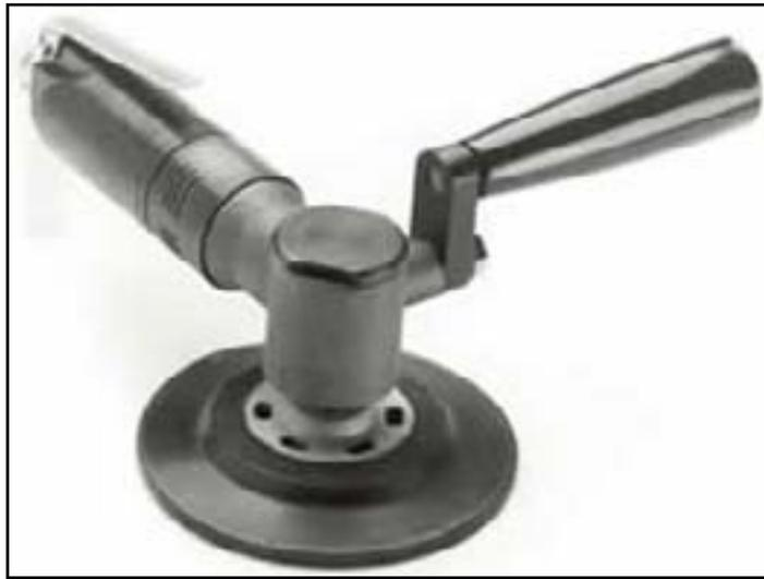
•This model can easily be adapted to a standard right angle grinder with the purchase of a wheel guard and appropriate grinding wheel adaptors.
