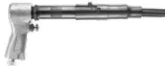
MODEL N-2RP PISTOL Needle SCALING HAMMER
